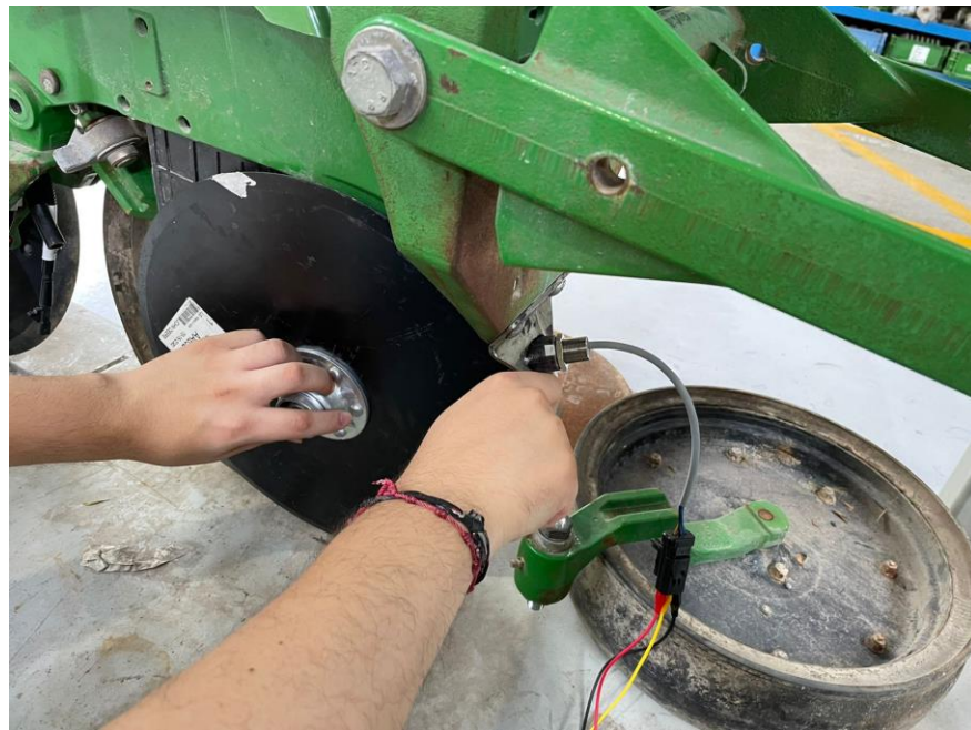
Figure A15. Picture detailing the testing process while spinning the disk
