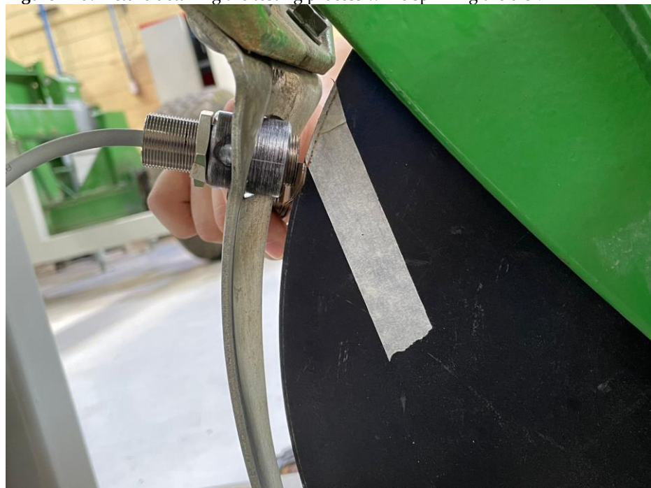
Figure A16. Picture detailing the measuring of real distance with feeler gauges.
