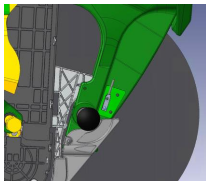
Figure A6. Location of the proposed second sensor that was discarded. The sensor would have different rivets in front of it at a distance of around 2mm.
